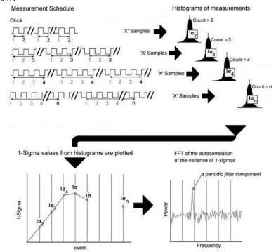
The highest frequency of the jitter spectrum is determined by the Nyquist frequency of the sampling interval. For accumulation in steps of one UI, the corresponding Nyquist frequency is one-half of the carrier frequency. The lowest frequency of the jitter spectrum is similarly determined by the longest span of UIs over which jitter is allowed to accumulate.
